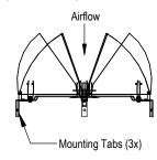
□ VCR8 - Steel full flow damper, duct mounted (sizes 10" to 14")
